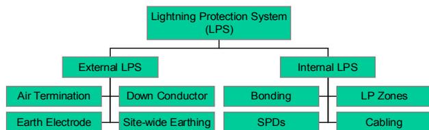
Figure 3: The Holistic Lightning Protection System
